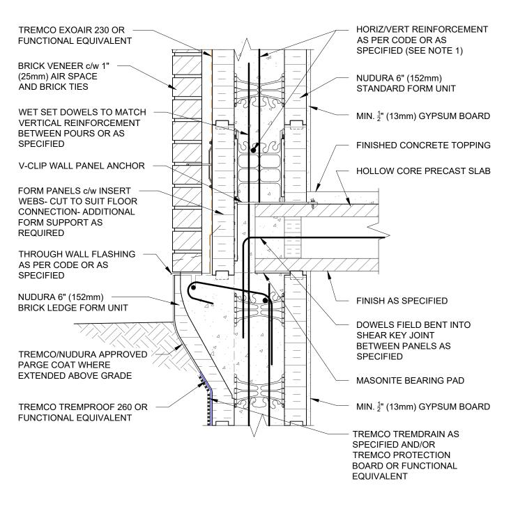
1) FOR OPTIMAL REINFORCEMENT PLACEMENT IN THE NUDURA FORM, SPACING OF HORIZONTAL REINFORCEMENT TO BE SPECIFIED AT 18" (457mm) O.C. AND VERTICAL REINFORCEMENT TO BE SPECIFIED AT MULTIPLES OF 8" (203mm) O.C. REFER TO NUDURA REINFORCEMENT PLACEMENT DETAILS.
